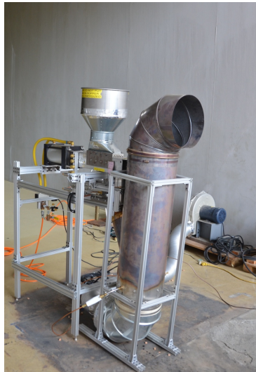
Fig. 7. Full scale continuous feed Firebrand Generator installed in BRI's FRWTF. The device is not producing firebrands at the time of this photograph.
