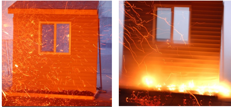
Fig. 3. In the image on left side, firebrands have caused smoldering ignition in the mulch bed [35]. In the image on the right side, smoldering ignition has transitioned to flaming ignition and the wall assembly has ignited. The dimensions of the wall assembly were 244 cm by 244 cm.
