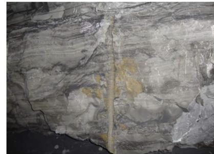
(c) Manual roof caving to form one side wall of the gateway.
