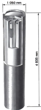
Fig.4. Copper-lined iron canister with channels for inserting bundles of spent fuel rods (After SKB).
