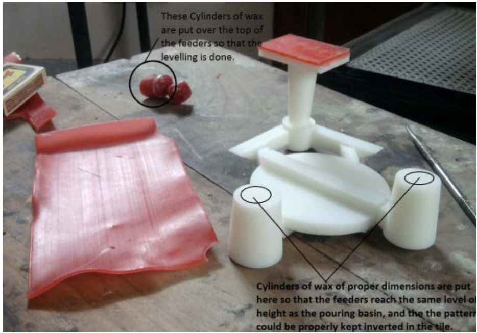
Figure 6. Balancing heights of pouring basin and risers with wax
