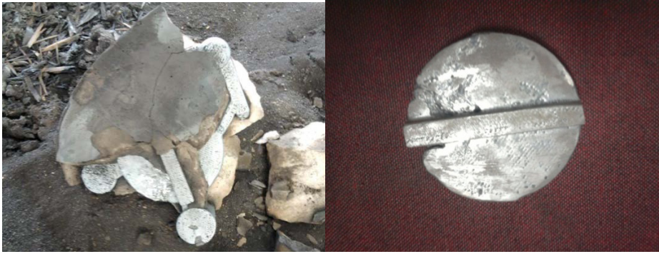
Figure 9. Pouring and then breaking the mould (left); Finished Cast using new Investment Casting (right)
