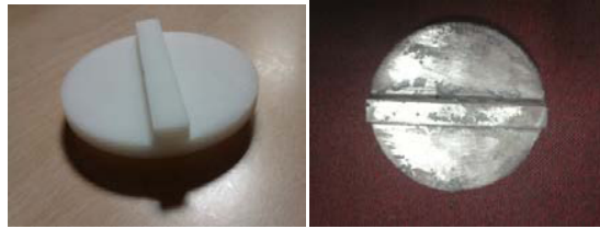
Figure 2. Pattern (left) and Cast Product (Right) for Sand Casting
