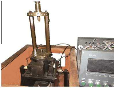
Fig. 8 Practical small-scale testing vibration mechanism.
