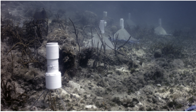
Fig. 2. Traps used in the second study. The lighted plankton trap, in the left foreground, stands on short legs—four large emergence traps can be seen in the middle-ground to the right of the lighted plankton trap. A second lighted plankton trap in the background can be seen towards the center of the frame.
