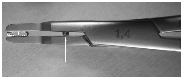
FIGURE 1. A clip applicator with a stopper within the jaw (white arrow) transforms the ligation clip into a rhombus with a shorter internal diagonal of 1.4 mm (indicated by white line).
