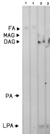
Fig. 2. Assessment of [ ^3\text{H} ]LPA metabolism. Membrane fractions were incubated with [ ^3\text{H} ]LPA (0.5 nM) for 60 min (see Fig. 1). The radioactive membrane lipids were extracted and separated on HPTLC plates (see Section 2). Lane 1 (run in duplicate) shows the methanol/water fraction and lane 2 (duplicate) the chloroform fraction.
