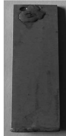
Fig. 8. Optical photo of the self-sealing pore film after salt spray test for 2000 h.
