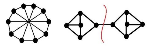
Fig. 1. The graph on the left has high conductance while the graph on the right has low conductance due to the "bottleneck" edge in the middle whose removal disconnects the graph. Both are 3-regular graphs on 10 nodes.
