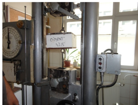
Fig. 2. Determination of tensile bond strength with the hydraulic press.
