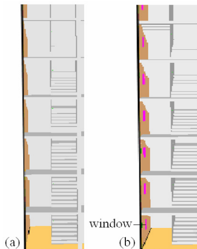
Fig 3 Staircase (a) without windows and (b) with opened windows
