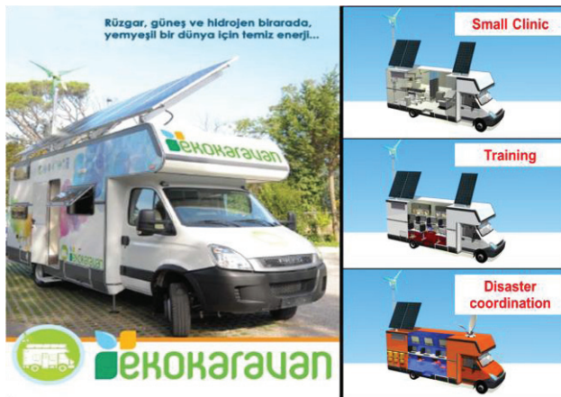
Fig. 6. Renewable-fuel cell energy demonstration mobile unit
