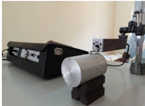
Figure 2: Measurement of surface roughness
