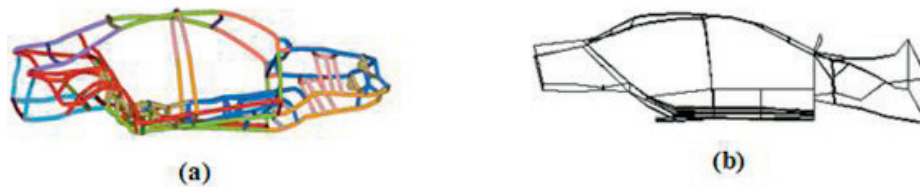
Fig. 7. Comparison of the BIW concept model torsion mode (a) with the torsion mode from the modal testing (b)
