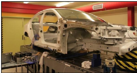
Fig 1: Experimental modal testing of the BIW
