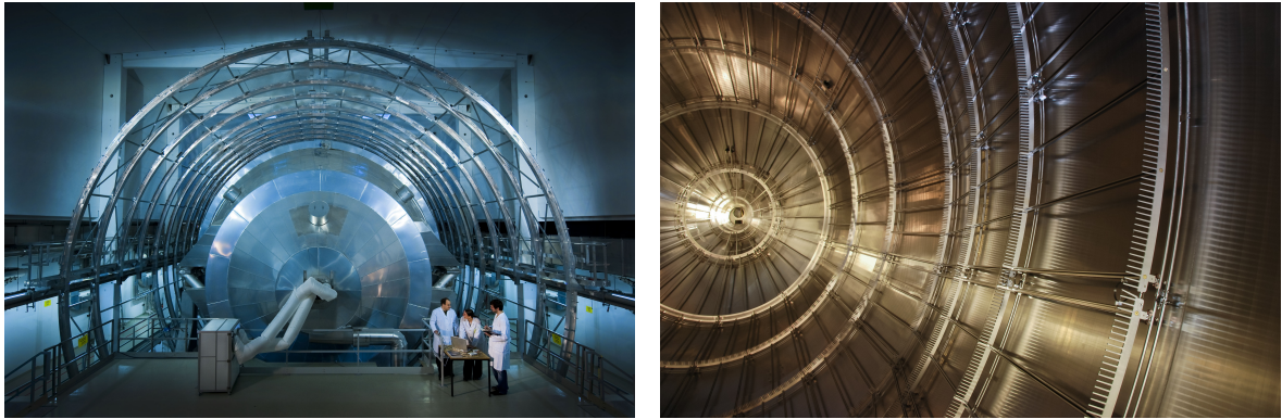
Figure 2. Left: The Air coil system consists of 3 sets of current loops distributed over a cylindrical surface around the main spectrometer. The 2 sets of axial loops compensate the 2 components of the earth magnetic field which are orthogonal to the spectrometer axis. The set of axial loops provide an axisymmetric correction field, which allows for precise adjusting of the magnetic field gradients and provides a magnetic field that prevents background electrons from penetrating the sensitive volume of the spectrometer. Right: The inner electrode system consists of more than 24 000 wires of a diameter of 300\ \mu\text{m} (outer layer) and 200\ \mu\text{m} (inner layer) at a distance of 15 cm (outer layer) and 22 cm (inner layer) to the surface of the main spectrometer tank. It serves as additional electric shielding against background electrons emitted from the tank wall as well as electric potential defining element.
