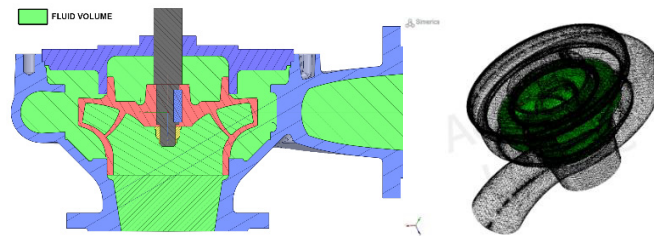
Fig.3: (a) CFD model fluid volume, (b) CFD model mesh
