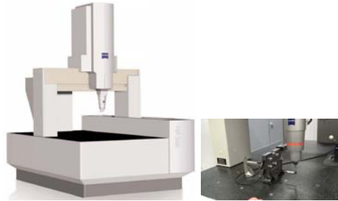
Fig. 1 - ZEISS Coordinate Measuring Machine, Model UPMC Ultra. The main specifications are: MPE (1/2D) = 0,3 + L/1000 \mu\text{m} , (with L mm) And MPE (3D) = 0,4 + L/1000 \mu\text{m} , (with L in mm).
