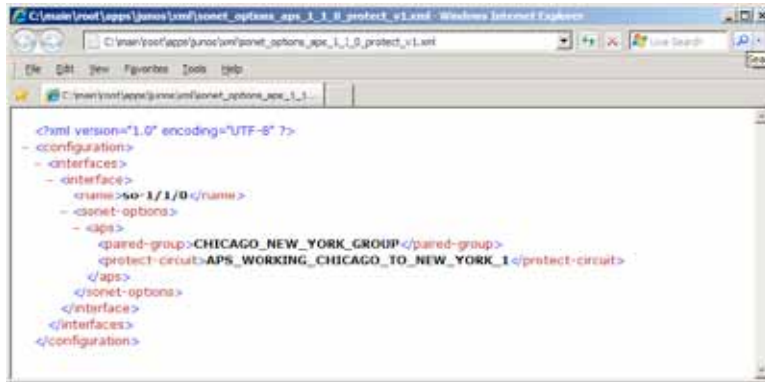
Fig. 2. Example JUNOS XML Fragment for SONET Automatic Protection Switching
