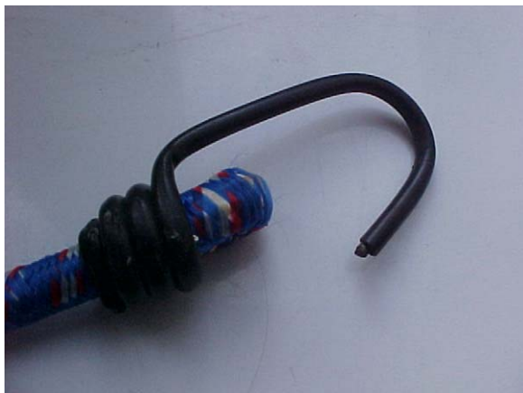
Figure 2 Typical metal hooked bungee cord. Although encased by rubber initially, repeated wear often exposes the sharp hook predisposing to lacerating as well as blunt injuries.
