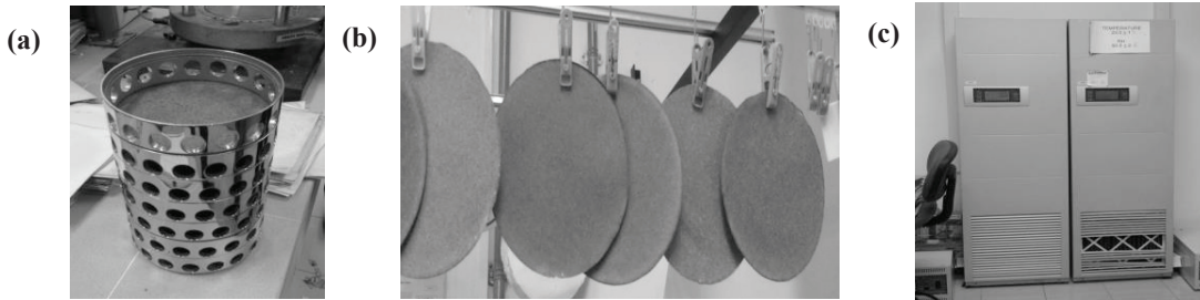
Fig. 6. (a) Dry ring (b) Durian rind CMP paper (c) Control room conditioning
