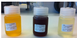
Figure 15. Aker Solutions' ACC™ advanced amine S26 solvent samples before and after reclaiming at TCM DA amine plant, and reclaimer waste (in the middle).
