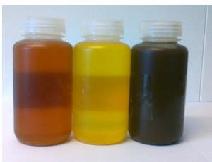
Figure 14. Aker Solutions' ACC™ advanced amine S21 solvent samples before and after reclaiming at TCM DA amine plant, and reclaimer waste.
