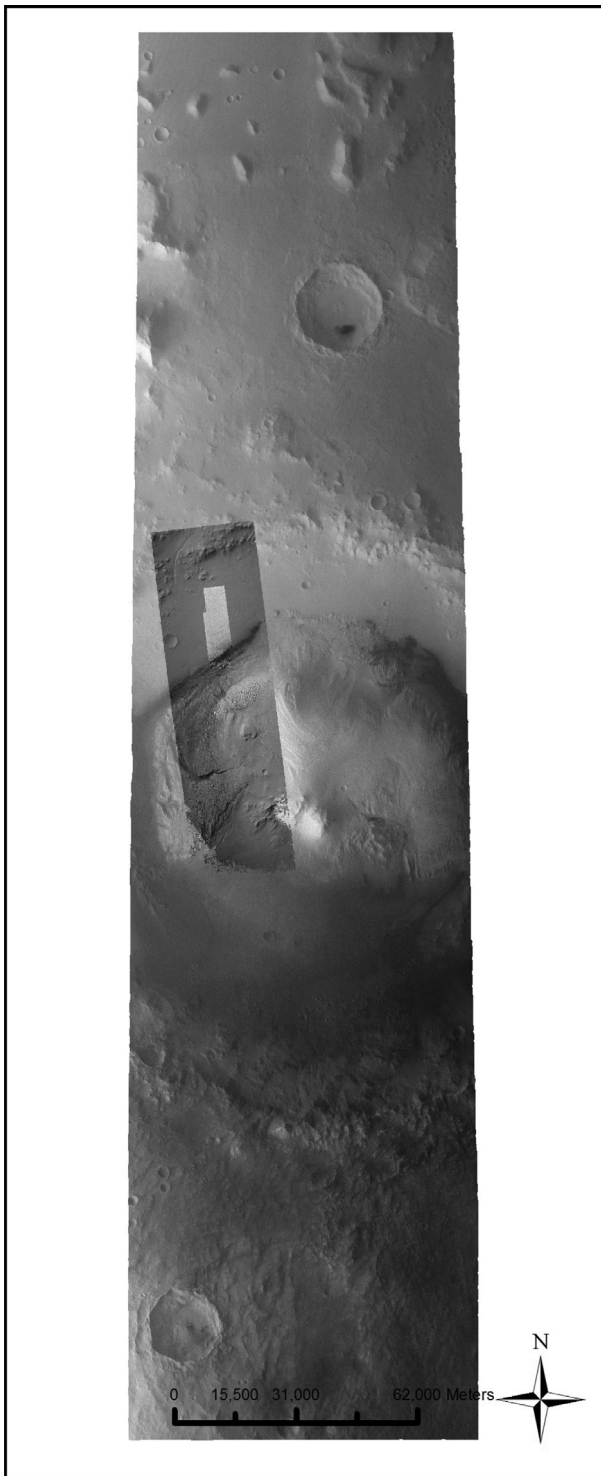
Fig. 30. The cascaded datasets created in this work for MSL showing co-registered HiRISE ORI on top of the CTX and HRSC ORI ( H1927_000_ND4 ) which is co-registered with MOLA.
