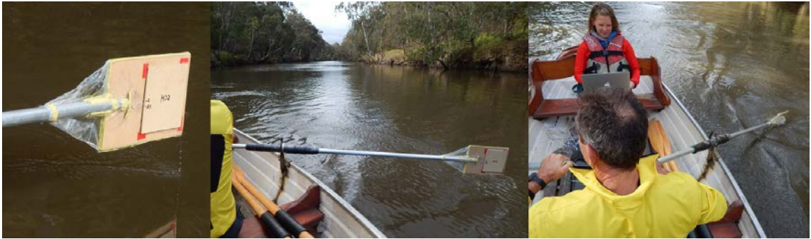
Fig. 3. smart blade used when rowing and recording of data
