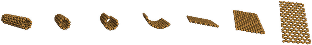
Figure 1: Snapshot sequence from an animation illustrating the unzipping of a carbon nanotube.
