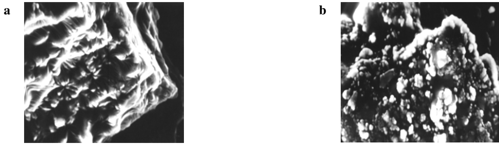
Fig. 5. Electronic micro-photographs of tar-polymeric binding agents (x3000) by composition: a – tar C_{30}^{10} = 215c with 1.5% of PVC, mineral powder of limestone is not activated; b – tar C_{30}^{10} = 215c with 1.5% of PVC, mineral powder of limestone is activated 0.5% of KF-MT.
