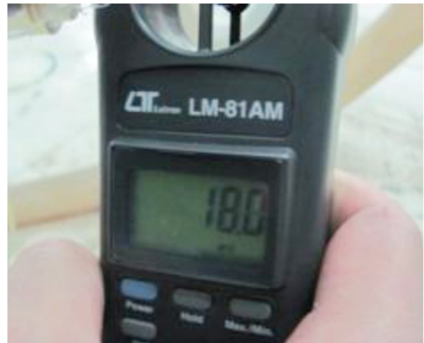
Figure 4: The anemometer showing injection air speed in each experiment.
