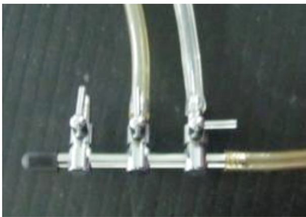
Figure 3: The division manifold that divides the main flow in three bottom hull injectors equally.
