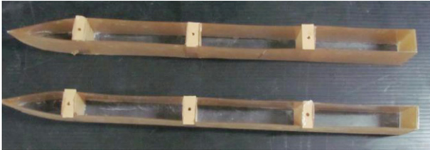
Figure 2: Plexiglass catamaran model with three separate injection chambers.
