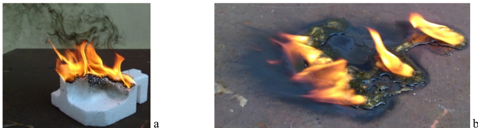
Fig. 2. Fire behavior of the polystyrene
