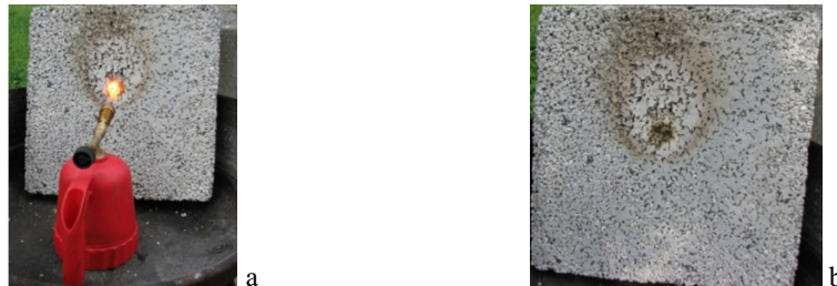
Fig. 4. Fire behavior of the polystyrene mortar
