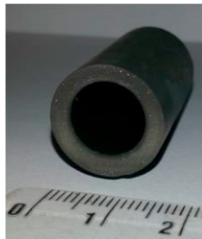
Fig. 3. Typical functionally graded hollow cylinder composites.
