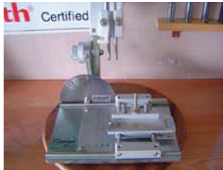
Fig. 2. Equipment of Loft and Lie Measurement
