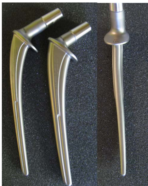
Figure 1 The chromium-cobalt Lubinus SP2™ stem has a double-curve anatomic form, providing a uniform cement mantle. The cervical angulation is 117°, with two neck lengths: standard and XL. Femoral offset and angulation are the same in all six of the sizes.
