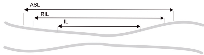
Fig. 1. Dose planning parameters in endovascular brachytherapy. IL (interventional length); ASL (active source length); RIL (reference isodose length)
