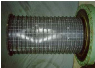
Fig. 2 Model failed by inelastic overall collapse.
