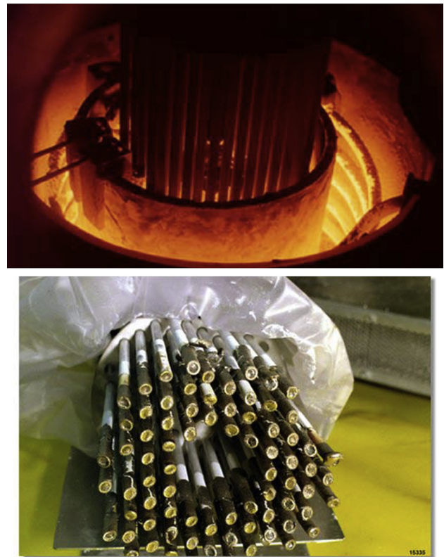
Fig. 1 – The full-length metallic Experimental Breeder Reactor (EBR)-II fuel in casting furnace (top) and after casting (bottom).
