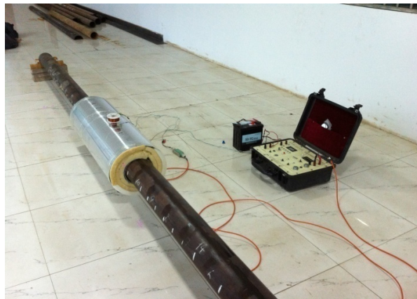
Fig. 3. PECT system in the pipe under insulation.
