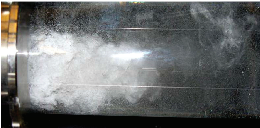
Fig. 6. 3D Steam condensation zone
