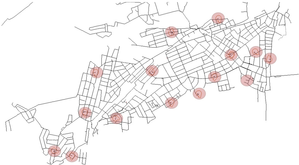
Fig. 7. Pumping stations in Zone 11.
