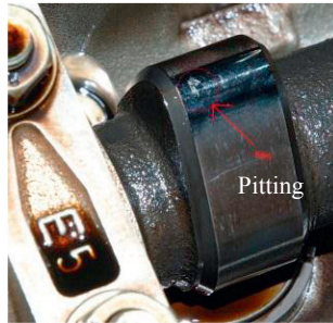
Fig 3: A camshaft lobe with surface wear [19].
