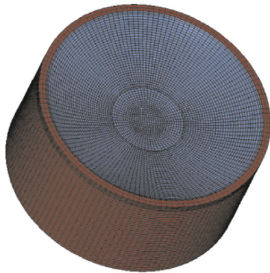
Fig. 5. Numerical modeling of EFP warhead.
