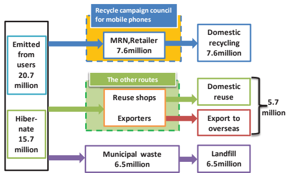
Fig.1 Basic material flow of used mobile phones
