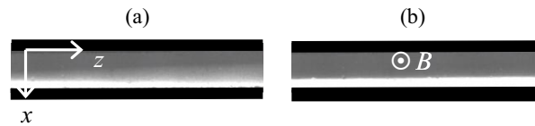
Fig. 2: Sharpening of the diffusion front upon application of the magnetic field. The flow rate is Q = 5 \mu\text{l}/\text{min} . (a) No magnetic field. (b) A homogeneous magnetic field of magnitude 3.5 mT is applied.
