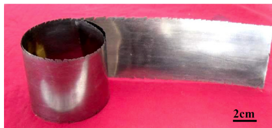
Fig. 5. Cold-rolled sheet of the Fe-6.5 wt%Si alloy composite slab (thickness: 0.2 mm).
