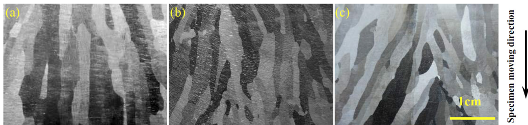
Fig. 3. Macrostructure of Fe-6.5 wt%Si alloy at inner part of slab at different withdrawing velocities for (a) 1 mm/min, (b) 2 mm/min and (c) 3 mm/min.
