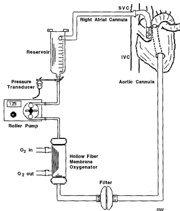
**Fig. 1.** CPB pump-oxygenator unit provides constant nonpulsatile flow and oxygenation through hollow-fiber membrane. Total volume of extracorporeal circuit is 46 ml. SVC, Superior vena cava; IVC, inferior vena cava.
