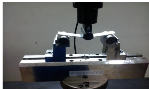
Figure 5. Three point bending with specimen
