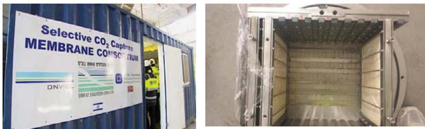
Fig. 4. a) DNV GL, NTNU & Yodfat Engineers Membrane Test Container b) The Membrane Unit
