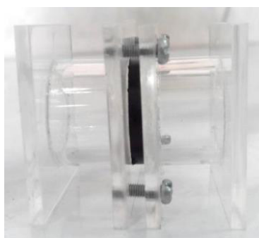
Fig. 1. The two-compartment chamber used for chemical polymerization of pyrrole inside the nanopores of AAO template.
