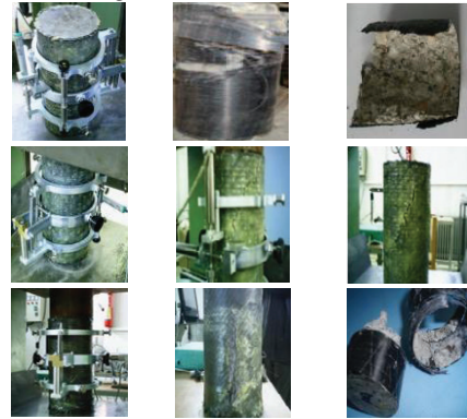
Fig. 18. Typical failure modes of CFRP-confined concrete cylinders
