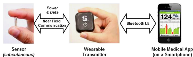
Fig. 1. Continuous glucose monitoring system components.
