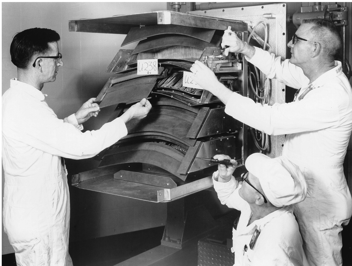
Figure 4. \beta unit collector assembly with labeled collector slits for one isotope pair. ORNL Photo 74250.
