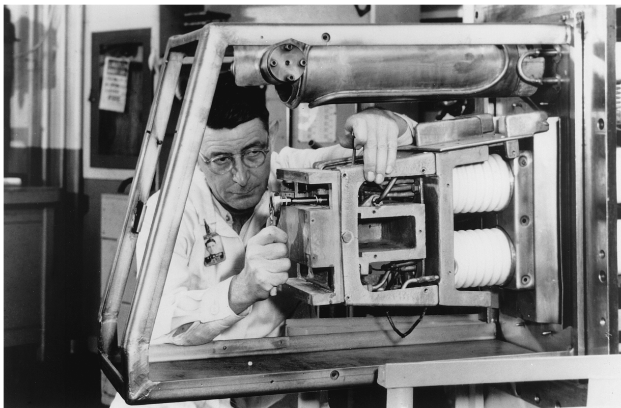
Figure 3. \alpha one calutron source showing charge box heater and two sets of filament heater ceramic standoffs. ORNL Photo 24574.
