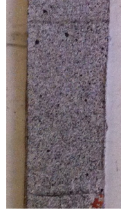
Fig. 3. Pattern on the specimen's area of interest.
